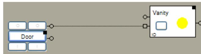
Finally the radio button-block has to be connected to the observer input pin (□) of the [switch actuator - block](#).
