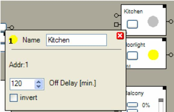
The switch actuator-block represents a real switch actuator within **myHomeControl**. It evaluates commands received from its preceding blocks. It generates radio message controlling the state of the corresponding real switch actuator.
