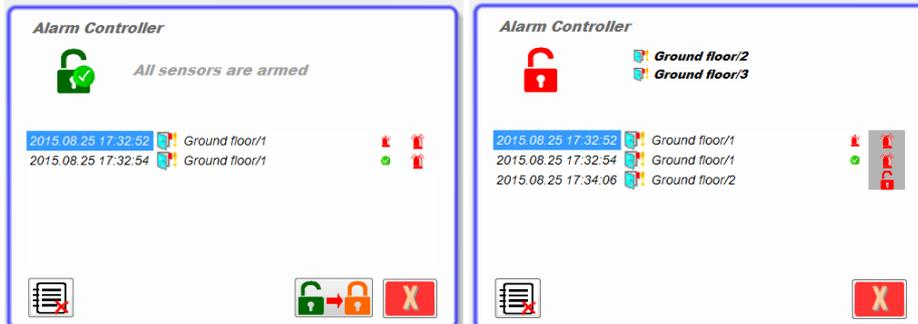
The upper left symbol shows the actual operation mode of the alarm controller.
