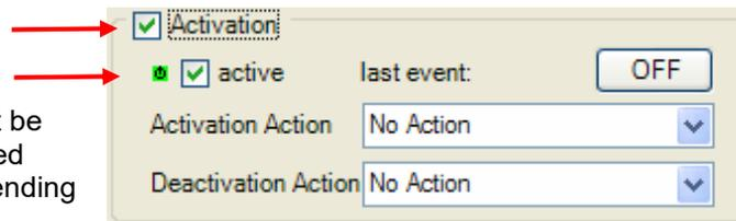
The button "last event" shows the stored last command the block has send or would have sent if it would be activated at the time the event appeared. A click on the button changes the type of command.
