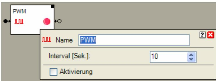
The Interval defines the rate for the generation of the pulses. This is the time between two pulses.
