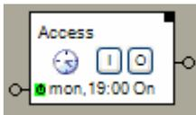
The clock is running and will process the list of given times. It will send commands at the corresponding times.
