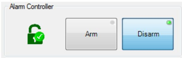
The symbol on the left side shows the actual operation mode of the alarm controller. Detailed information will be shown if the symbol is clicked.
