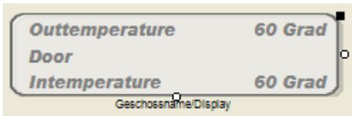
All the signals connected to the block in the network area are shown by this visualization element. The displayed names and units can be configured within the properties dialog of the network block.
