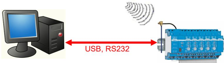
Via this connection **myHomeControl** will receive all radio messages received by the antenna module of the bus system as well as all radio messages received by a subantenna. Also all feedback messages of the various actuators as well as sensor directly connected to the bus will be forwarded to **myHomeControl**.
