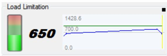
Power consumption level is below the limit. The consumption is shown as a trend:
