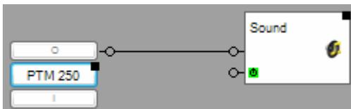
In case the I button has been pressed the block plays the audio file assigned to the ON event. In case the O button has been pressed the block plays the audio file assigned to the OFF event.
