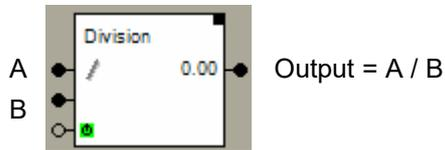
In case  $B = 0$ , then the value of the output becomes the maximal positive value.
